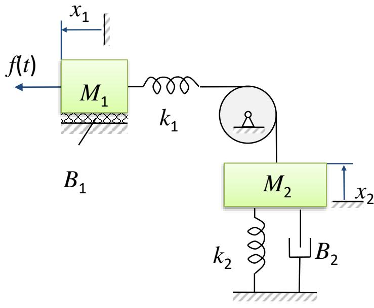
$$\begin{array}{c} f(t) \leftarrow \\ M_1 \xrightarrow{\quad} \end{array} \begin{array}{l} B_1 \dot{x}_1 \\ M_1 \ddot{x}_1 \end{array} \xrightarrow{\quad} \begin{array}{l} B_1 \dot{x}_1 \\ k_1(x_1 - x_2) \end{array}$$
