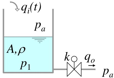
$$\left. \begin{aligned} \dot{p}_1 &= \frac{1}{C} [q_{in}(t) - q_{out}(t)] \\ q_{in}(t) &= q_i(t) \\ q_{out}(t) &= k\sqrt{p_1 - p_a} \end{aligned} \right\} \dot{p}_1 = \frac{1}{C} [-k\sqrt{p_1 - p_a} + q_i(t)]$$
